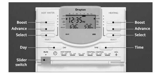
The Tempus 6 electronic programmer will automatically switch ON and OFF up to three times a day. You can select one set of times for weekdays and different times for weekends (5/2 day), or programme each day of the week the same (24 hour). Hot water and heating times can be set independently.
