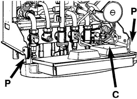
from spark generator. Loosen screws securing the closure plate and remove. Remove grommet from base of sealed chamber. Remove screw securing electrode bracket and lift clear easing spade connectors through the grommet. Reassemble in reverse order, twisted together electrodes cable at least 10 times to avoid electrical interference.
