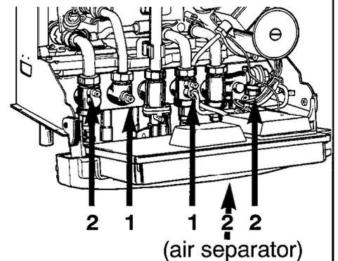
1 = DHW circuit drain point
