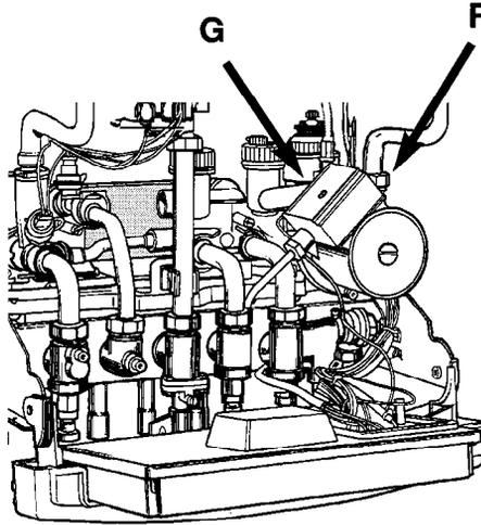
the clip (G) on the pump volute and pull pump toward you. Reassemble in reverse order.
