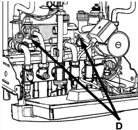
Prior to reassembly, check that the 4 gaskets are correctly positioned. The heat exchanger is so designed that it cannot be remounted incorrectly.
