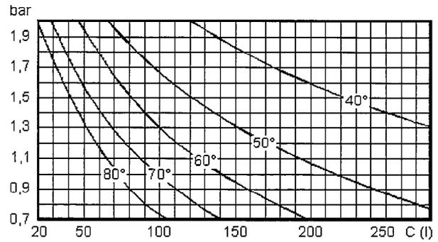
Note : The system initial pressure should be over the following value :
