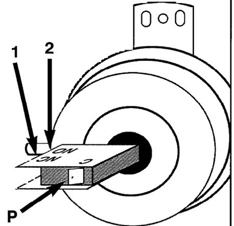
P = orange cable connected to C
