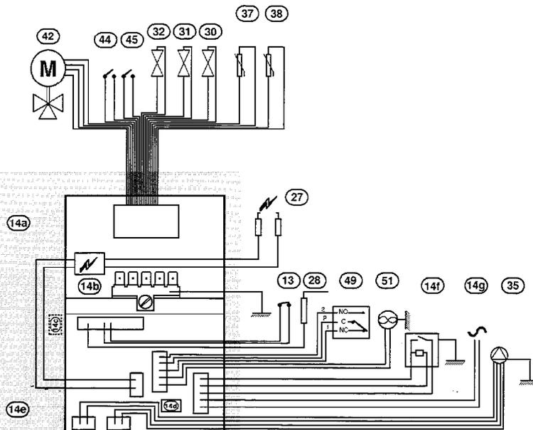
**Plug for main power and Room thermostat connection**
