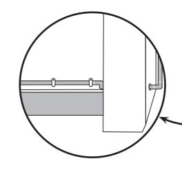
Additional Note: take care to prevent **brick dust** entering pipe when pushing the pipe through the wall
