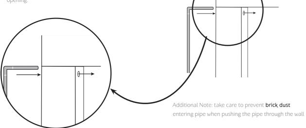
Push the condensate pipe supplied into the builder's opening through the drilled hole and connect the pipe to the plastic elbow.
