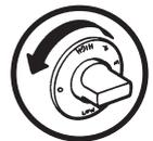
**To switch the boiler off. (Electronic Controls Boiler)** Turn the thermostat knob to the OFF position (●).
