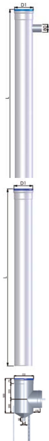
T-PIECE 1 CONNECTION Ø 80 Ø 130 L=1550
