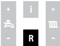
The reset key restarts the boiler after a malfunction has occurred.
