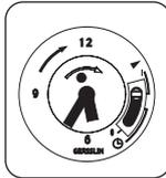
1. **Position "1" CONSTANT:** in this position, the clock circuit is always closed (switch on), therefore the boiler will constantly be on and will only shut off upon the request of the room thermostat (if installed) or the heating thermostat;
