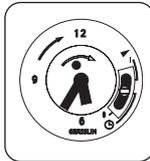
3. **"Central" Position PROGRAMMING ACTIVE:** in this position, the programming set by the user is active.
