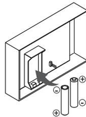
Ensure the batteries (2 x 1.5V L26/AA) are correctly fitted
