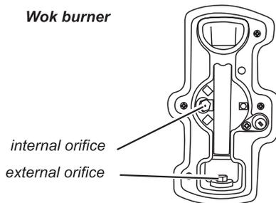
Remove burner cap and head. Remove old jet. Fit new orifice. **Note** the Wok burner has 2 orifices. Reassemble in reverse order. Check appliance is gas sound.
