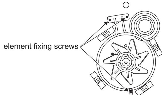
Remove the fixings that secure the element within the oven and lift the element away carefully. Disconnect the leads and connect to the replacement element and re-assemble parts in reverse order. Check that the oven operates correctly.
