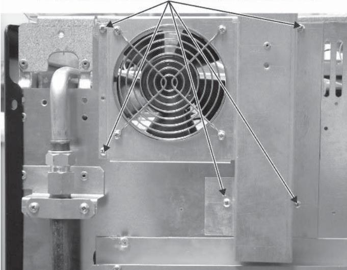
Support the fan and remove the screws holding the cooling fan mounting bracket. Gently lift the fan and bracket away from the range taking care not to strain the electrical connection. Disconnect the leads from the fan noting the orientation. Remove the fan from the mounting bracket. Fit the new fan and reassemble in reverse order.
