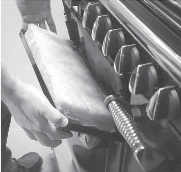
Reassemble in reverse order making sure that the pad of insulation is in place.
