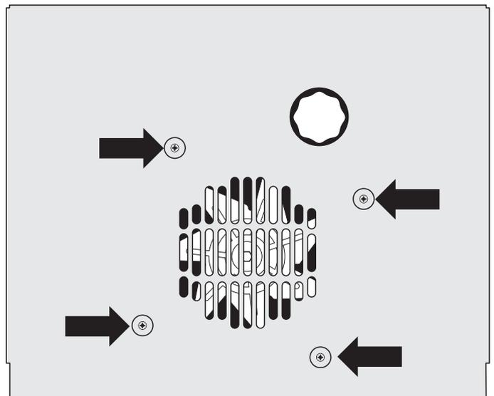
Remove the fixings that secure the inner back to the oven rear. Lift the removable panel away. Re-assemble in reverse order. Ensure that the retaining fixings are fully tightened. For the LH oven unscrew the 2 thermostat phial fixing screws. Remove the screws that secure the inner back to the oven rear. Lift the removable
