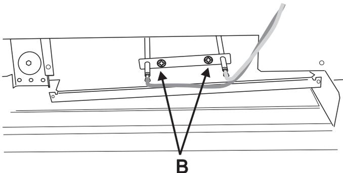
Remove the 2 screws B, holding the element to the bottom sheet..
