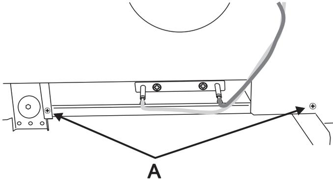
Remove the 2 screws 'A' and allow the plate to drop down.
