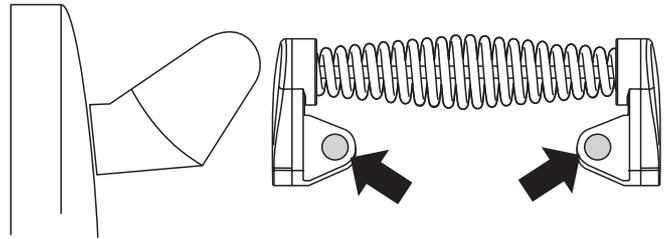
Remove the two plastic blanking plugs from the door handles. Remove the 4mm Hex headed screws holding the handle to the door with the hexagon key tool. Remove two screws from top edge and two from bottom edge of the door.
