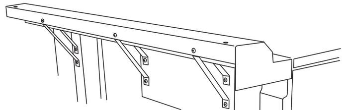
Remove the screws holding the flue grille stays and if the rear extension is fitted remove the screws holding that as well.
