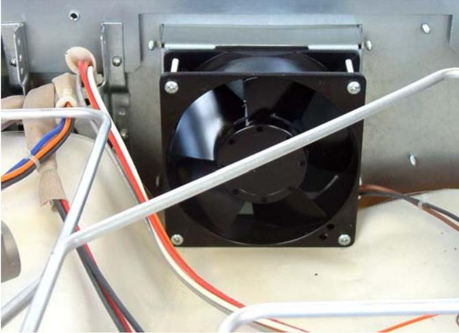
Disconnect the leads from the fan noting the orientation. Remove the fan from the mounting bracket. Fit the new fan and reassemble in reverse order.
