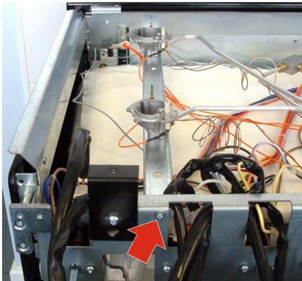
Remove the screw at the front holding the cross support. Slide the support to the right to release it from the rear location. Lift the cross support and burners clear. The burners are fixed to the cross supports with screws underneath. Remove the appropriate burner and fit the new one. Reassemble in reverse order. Check burner operation is satisfactory.
