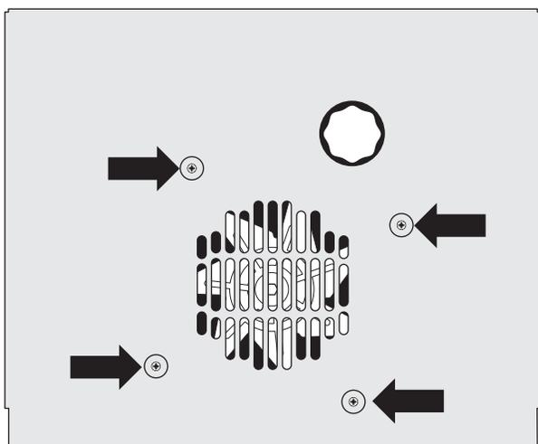
Remove the fixings that secure the inner back to the oven rear.
