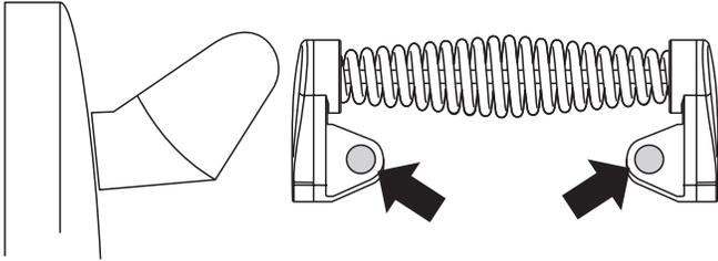
Remove the two plastic blanking plugs from the door handles. Remove the 4mm Hex headed screws holding the handle to the door with the hexagon key tool. Remove two screws from top edge and two from bottom edge of the door. Remove outer door panel. Fit door handle to new panel. Fit the plastic blanking plugs to the fixing holes.
