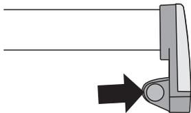
Remove the handrail plastic blanking plugs and remove the 2 end bracket fixing screws.
