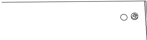
Open the broiler door and R H oven door and remove the 2 screws underneath the control panel.
