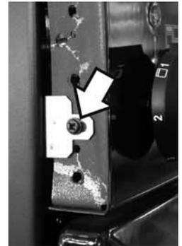
Remove the retaining screws for each panel (1 at the front and 2 at the rear). The lower front retaining screws (one each side) are situated beneath the lower edge at the front corners of the side panels
