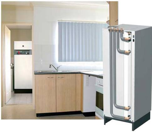
The HeatMaster 35 TC can be installed with the optional easy-fit manifold kit incorporating 22mm compression fittings, which allows all the hot, cold and heating pipework to be connected easily and conveniently at the top of the HeatMaster TC. The easy-fit kit enables the HeatMaster 35 TC to be installed into a confined space whilst still giving access to the pipework connections.
