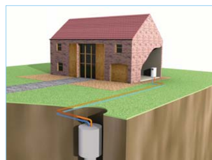
Bore hole collector
