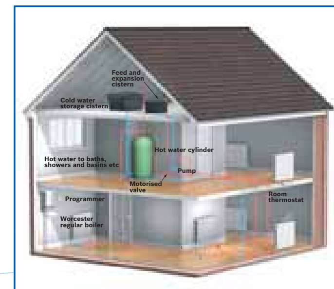
How a Greenstar condensing regular system fits into your home.
