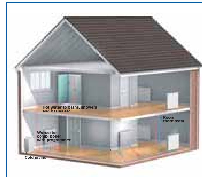
How a Greenstar condensing combi system fits into your home.
