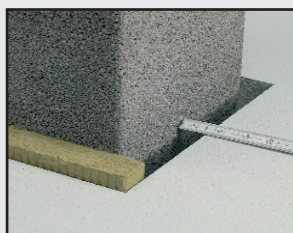
Leave a gap of 40mm at ceiling / floors. Fill this gap with a non-combustible material.
