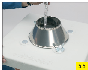
5.5 Place the cone and measure the missing pipe length.
