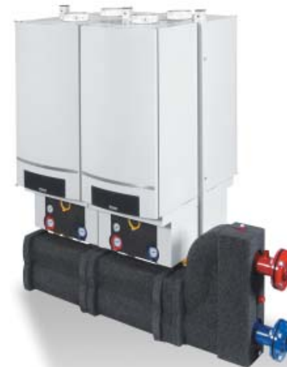
GB162 four boiler back-to-back cascade with up to 400 kW in 1m 2 . Boilers shown with Buderus pump groups and the full cascade kit.
